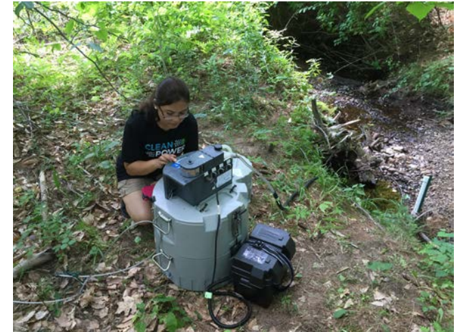
Setting ISCO sampler to catch storm event
